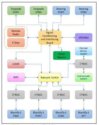
Figure 10 Computer System Block Diagram
