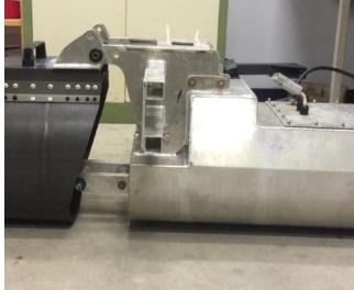
Figure 5: Floatation pod design used in the 2016 competition. A large void is present between the rear of the WAM-V pontoon and the floatation pod which produced large drag forces when underway.
