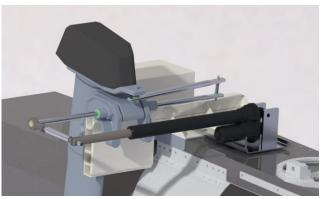
Figure 6 Linear-Actuator Based Steering System
