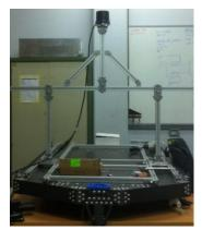
Figure 4: The Antenna Mast mounted to the Modular Rail System allowing adjustment to position without drilling new mounting holes in the WAM-V payload tray.
