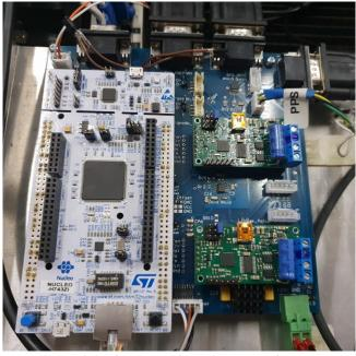
Figure 9 Signal Conditioning and Interfacing Board
