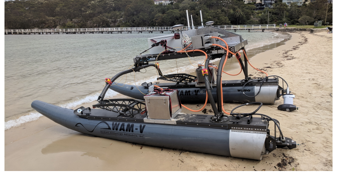
Fig. 5. The WAM-V on field test day 2, flotation pods detached
